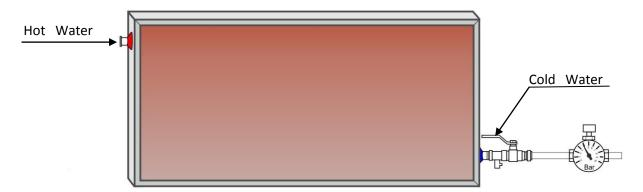
1. Connect the safety valve at the cold water inlet.
