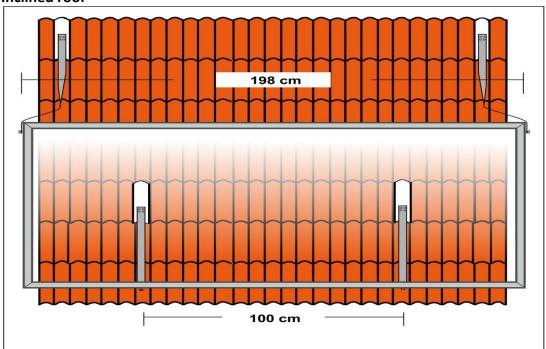
1. Affix the top and bottom collector straps to the beams under the roofing material.
