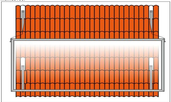
1. Affix the top and bottom collector straps to the beams under the roofing material.
