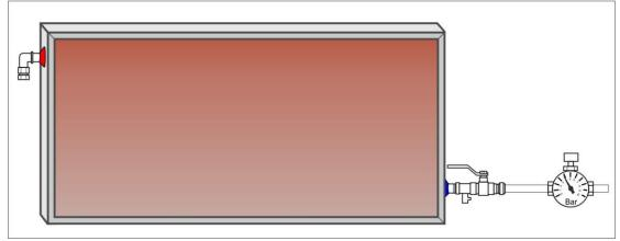
1. Connect the safety valve at the cold water inlet.
